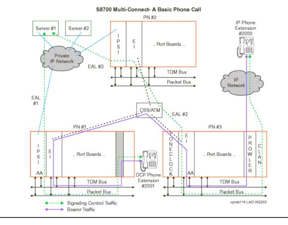
**IP Server Interface (TN2312BP) -** The IP Server Interface (IPSI) is the communication interface between the server and the Media Gateways (port networks). The IPSI is responsible for gateway control, and for tunneling call control messages back to the S8700.
